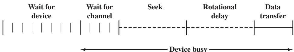
Figure 6.5 Timing of a Disk I/O Transfer
