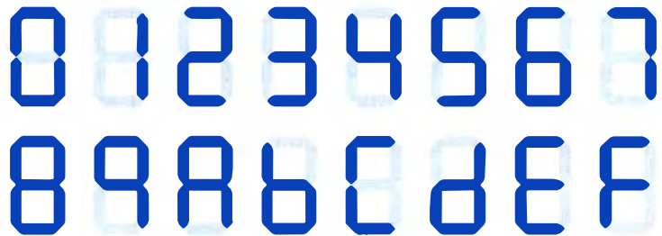
Figure Ex. 4.30 Specification for the 7-segment display of hexadecimal digits.
