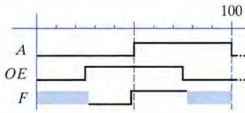
Figure 4.49 Waveform with a high-impedance output.
