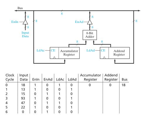
**12.40** A digital system can perform any four-variable bitwise logic function, but it may take several clock cycles. (A bitwise logic function performs the same logic function on each bit.) Recall that the NAND operation is functionally complete (i.e., we can do any logic function by a series of NAND operations). On the following 8-bit registers, En is a tristate buffer enable as in Figure 12-3, and CE is a clock enable as in Figure 12-1.
