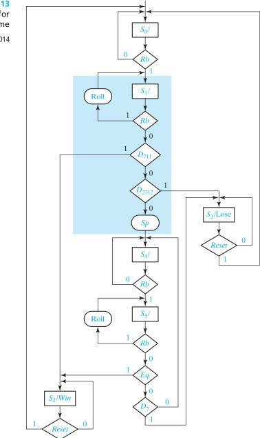
We can now convert the flowchart for the dice game to an SM chart for the control circuit using the defined control signals. Figure 19-13 shows the resulting SM chart. The control circuit waits in state  $S_0$  until the roll button is pressed (Rb = 1). Then, it goes to state  $S_1$ , and the roll counters are enabled as long as Rb = 1. As soon as the roll button
