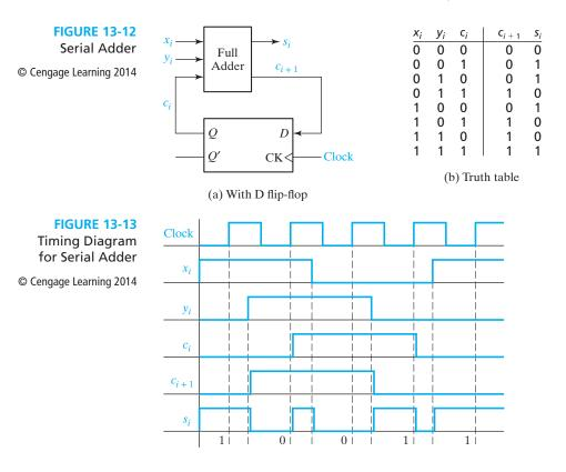
and  $c_2 = 1$ , which is stored in the flip-flop on the rising clock edge. This process continues until the addition is completed. Reading the sum output just before the rising edge of the clock gives the correct result.
