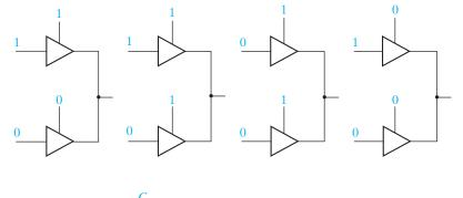
(d) The symbol represents 2 three-state buffers with a common  $A \xrightarrow{2} B$  control input:
