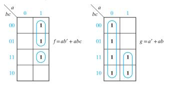
In each case, change the looping on the map so that the minimum solution is obtained.
