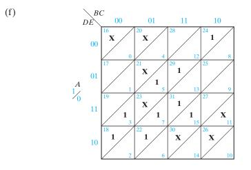
Find the three 1's and X's adjacent to  $1_{18}$ . Can these all be looped with a single loop?
