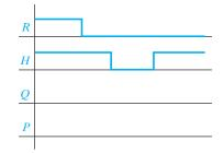
**11.3** This problem illustrates the improper operation that can occur if both inputs to an S-R latch are 1 and are then changed back to 0. For Figure 11-6, complete the following timing chart, assuming that each gate has a propagation delay of exactly 10 ns. Assume that initially P = 1 and Q = 0. Note that when t = 100 ns, S and R are both changed to 0. Then, 10 ns later, both P and Q will change to 1. Because these 1's are fed back to the gate inputs, what will happen after another 10 ns?
