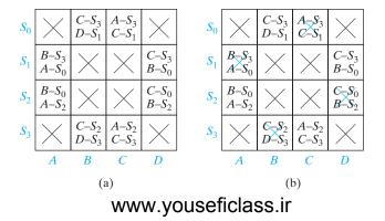
Similarly, square B- $S_3$  is crossed out because  $C \neq S_2$ , square C- $S_0$  because  $A \neq S_3$ , and square D- $S_2$  because  $B \neq S_2$ . Another pass through the table reveals no additional nonequivalent pairs; therefore, the remaining equivalent state pairs are
