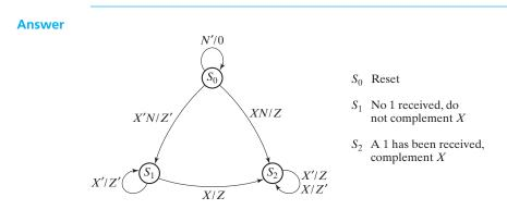
The counter will generate a completion signal (K) when it reaches state 15. Modify your state graph so that when K = 1, the circuit will complete the 2's complement operation and return to the initial state. Also, add the *Sh* output in the appropriate places.
