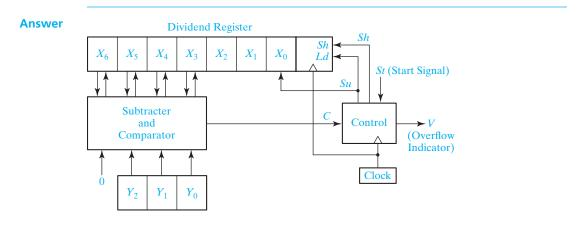
If the contents of the dividend register is initially 0100010 and the divisor is 110, show the contents of the dividend register after each of the first three rising clock edges. Also, indicate whether a shift or a subtraction should occur next.
