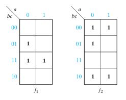
(d) Find expressions which correspond to a two-level, minimum multipleoutput, AND-OR realization of  $F_1$ ,  $F_2$ , and  $F_3$ . Why should the term *cd not* be included in  $F_1$ ?
