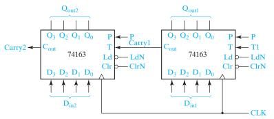
The 74163 (see Figure 17-12) is a 4-bit fully synchronous binary counter which is available in both TTL and CMOS logic families. Although rarely used in new designs at present, it represents a general type of counter that is found in many CAD design libraries. In addition to performing the counting function, it can be cleared or loaded in parallel. All operations are synchronized by the clock, and all state changes take place following the rising edge of the clock input.
