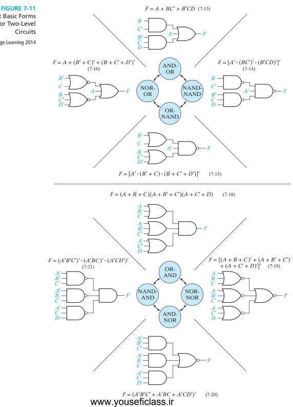
**Eight Basic Forms** for Two-Level © Cengage Learning 2014 Equations (7-18), (7-19), (7-20), and (7-21) represent the OR-AND, NOR-NOR, AND-NOR, and NAND-AND forms, respectively, as shown in Figure 7-11. Two-level AND-NOR (AND-OR-INVERT) circuits are available in integrated-circuit form. Some types of NAND gates can also realize AND-NOR circuits when the so-called *wired OR* connection is used.
