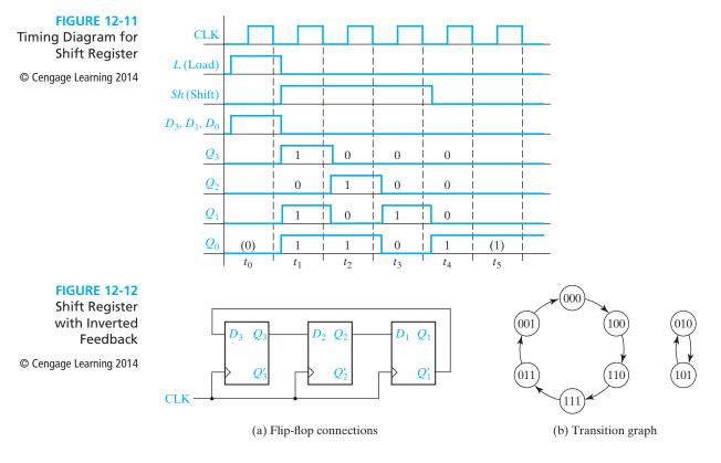
the register is in state 001,  $D_3$  is 0, and the next register state is 000. Then, successive clock pulses take the register around the loop again. Note that states 010 and 101 are not in the main loop. If the register is in state 010, then a shift pulse takes it to 101 and vice versa; therefore, we have a secondary loop on the transition graph.
