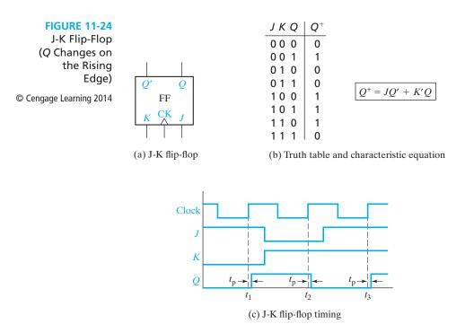
from 1 to 0. The next-state table and characteristic equation for the J-K flip-flop are given in Figure 11-24(b).
