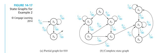
If we receive a 1 in state  $S_6$ , the 010 sequence is broken and we must add a new state  $(S_7)$  to start looking for 010 again. In state  $S_7$  we ignore additional 1's, and when a 0 is received, we go back to  $S_5$  because this 0 starts the 010 sequence over again. Figure 14-17(b) shows the complete state graph, and the corresponding table is Table 14-6.
