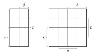
Two alternative forms for five-variable maps are used. One form simply consists of two four-variable maps side-by-side as in Figure 5-28(a). A modification of this uses a *mirror image* map as in Figure 5-28(b). In this map, first and eighth columns are "adjacent" as are second and seventh columns, third and sixth columns, and fourth and fifth columns. The same function is plotted on both these maps.
