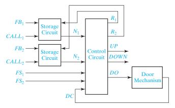
signal  $N_i$  is stored so that a single pulse on  $FB_i$  or  $CALL_i$  will set  $N_i$  to 1 until the control circuit clears it, then the control circuit will be simplified further. Using a D flip-flop and a minimum number of added gates, design a storage circuit that will have an output 1 when either input ( $FB_i$  or  $CALL_i$ ) becomes 1 and will stay 1 until reset with a signal  $R_i$ .
