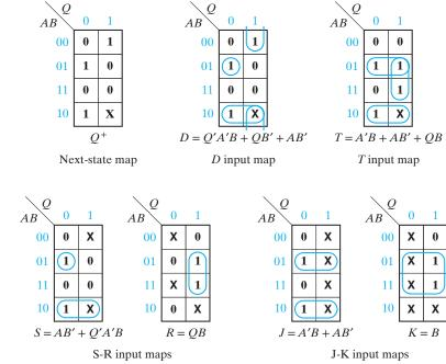
For the S-R flip-flop, note that when Q = 0, R = X if  $Q^+ = 0$ ; and when Q = 1, R = 1 if  $Q^+ = 0$ . Therefore, to form the R map from the  $Q^+$  map, replace 0's with X's on the Q = 0 half of the map and replace 0's with 1's on the Q = 1 half (and fill in 0's for the remaining entries). Similarly, to form the S map from the  $Q^+$  map, copy the 1's on the Q = 0 half of the map, and replace the 1's with X's on the Q = 1 half.
