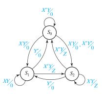
**15.36** A state graph for a single-input sequential circuit is given. Implement the circuit using a three-bit parallel loading counter that has the given operation table. Label the counter outputs  $Q_2$ ,  $Q_1$ ,  $Q_0$ , where  $Q_0$  is the least significant bit and the parallel inputs  $P_2$ ,  $P_1$ ,  $P_0$ . (*Hint:* Because the Ld signal overrides the Cnt signal, the counting sequence can easily be changed by doing a parallel load at the appropriate times.)
