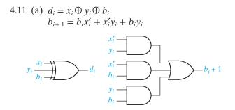
(b)  $d_i = s_i, b_{i+1}$  is the same as  $c_{i+1}$  with  $x_i$  replaced by  $x'_i$ 4.12
