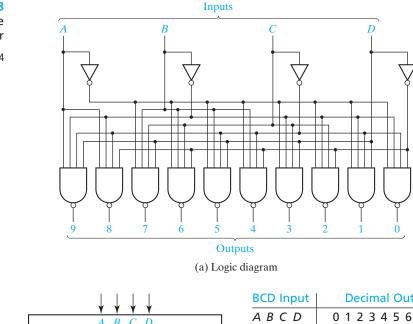
FIGURE 9-18 A 4-to-10 Line Decoder
