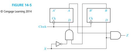
The procedure for finding the state graph for a Moore machine is similar to that used for a Mealy machine, except that the output is written with the state instead of with the transition between states. We will rework the previous example as a Moore machine to illustrate this procedure. The circuit should produce an output of 1 only if an input sequence ending in 101 has occurred. The design is similar to that for the
