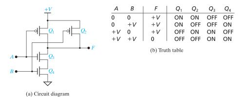
Figure A-6 shows a CMOS NOR gate. If A = 1 (+V),  $Q_1$  is off and  $Q_4$  is on, F = 0. Likewise, if B = 1,  $Q_2$  is off and  $Q_3$  is on, so F = 0. Because F = 0 when A or B is 1, F' = A + B, and F = (A + B)', which is the NOR function.
