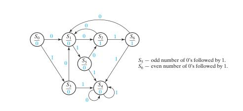
Verify that this state graph gives the proper output sequence for each input sequence at the start of this exercise. Write down the Moore state table which corresponds to the preceding graph. (Note that a Moore table has only one output column.)
