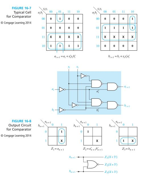
For the output circuit, let  $Z_1 = 1$  if X < Y,  $Z_2 = 1$  if X = Y,  $Z_3 = 1$  if X > Y. Figure 16-8 shows the output maps, equations, and circuit.
