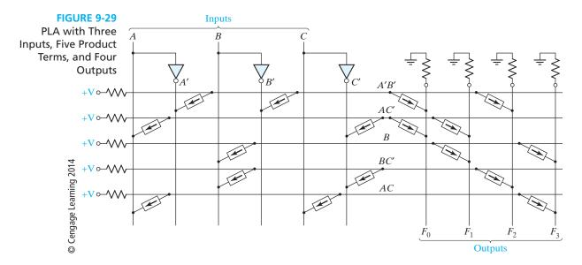
Switching elements are connected in the OR array to select the product terms needed for the output functions. For example, because  $F_0 = A'B' + AC'$ , switching elements are used to connect the A'B' and AC' lines to the  $F_0$  line. The connections in the AND and OR arrays of this PLA make it equivalent to the AND-OR array of Figure 9-30.
