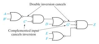
(b) Equivalent circuit with NOR gates
