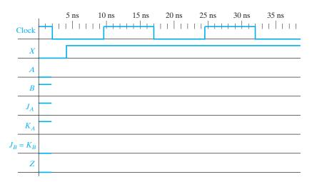
**13.29** Draw a timing diagram for the following circuit starting with an initial state ABC = 000 and using an input sequence X = 01010. Assume that the input changes occur midway between the falling and rising clock edges. Give the output sequence, and indicate false outputs, if any. Verify that your answer is correct by making a state table for the circuit.
