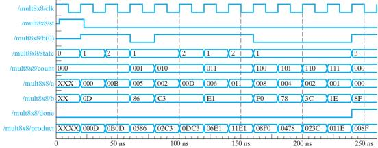
Figure 20-10 shows a simulator command file used to test the multiplier with inputs  $11 \times 13$ . The A and B register values and the product are shown in hexadecimal on the resulting waveforms. The current multiplier bit (M) is the same as b(0). Note that at time = 240 ns, the state changes to 3, the Done signal is turned on, and the final product is the correct answer,  $8F_{16} = 143_{10}$ .
