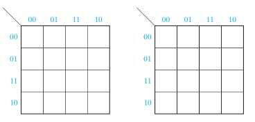
(b) Plot the map for the output function (Z) from the transition table of Table 15-9(b) and derive the minimum equation for Z.
