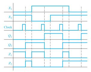
**13.24** Given the following timing chart for a sequential circuit, construct as much of the transition table as possible.
