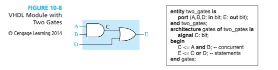
When we describe a system in VHDL, we must specify an entity and an architecture at the top level, and also specify an entity and architecture for each of the component modules that are part of the system (see Figure 10-9). Each entity declaration includes a list of interface signals that can be used to connect to other modules or to the outside world. We will use entity declarations of the form:
