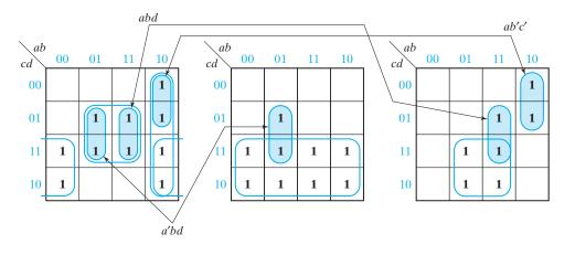
By inspecting the maps, we can see that terms a'bd (from  $f_2$ ), abd (from  $f_3$ ), and ab'c' (from  $f_3$ ) can be used in  $f_1$ . If bd is replaced with a'bd + abd, then the gate needed to realize bd can be eliminated. Because  $m_{10}$  and  $m_{11}$  in  $f_1$  are already covered by b'c, ab'c' (from  $f_3$ ) can be used to cover  $m_8$  and  $m_9$ , and the gate needed to realize ab' can be eliminated. The minimal solution is therefore
