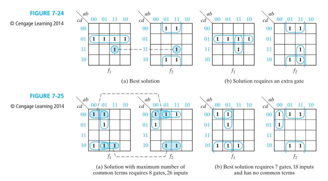
appears on the  $f_2$  map. In Figure 7-25, the only minterms of  $f_1$  which do not appear on the  $f_2$  map are  $m_2$  and  $m_5$ . The only prime implicant which covers  $m_2$  is a'd'; hence, a'd' is essential to  $f_1$  in the multiple-output realization. Similarly, the only prime implicant which covers  $m_5$  is a'bc', and a'bc' is essential. On the  $f_2$  map, bd' is essential. Why?
