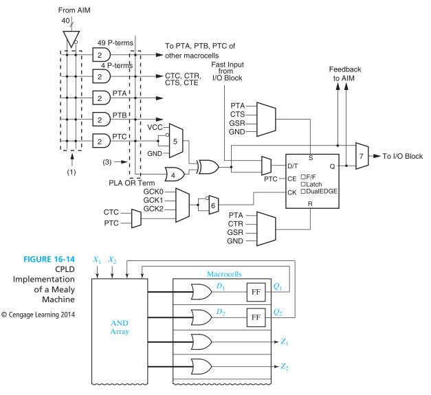
to generate the D inputs to the flip-flops and two to generate the Z outputs. The flip-flop outputs are fed back to the AND array inputs via the interconnection matrix (not shown). The number of product terms required depends on the complexity of the equations for the D's and the Z's.
