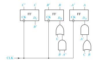
An alternative to directly designing counters for nonbinary sequences is to use a binary counter or some other counter and add decoding logic to generate the
