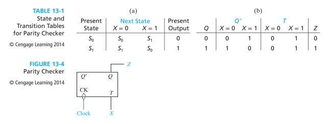
flip-flop to the proper initial state (Q = 0) before checking the parity of another input sequence.
