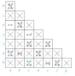
this point whether or not  $a \neq d$ . Similarly, because neither square *b*-*d* nor *c*-*h* contains an X, we cannot determine immediately whether  $a \neq g$  or not. Going on to the second column, we place X's in squares *b*-*d* and *b*-*g* because we have already shown  $a \neq f$  and  $b \neq f$ . In a similar manner, we check each of the remaining columns and X out squares *c*-*f*, *d*-*g*, *e*-*f*, and *f*-*h*. Figure 15-4 shows the resulting chart.
