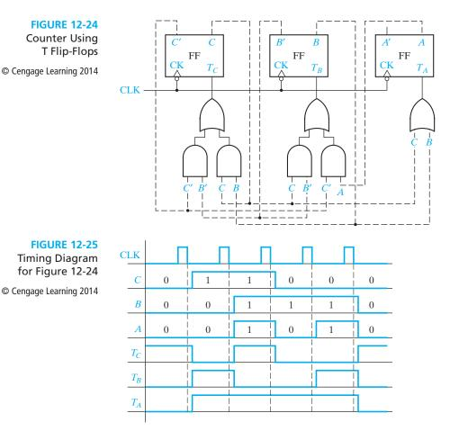
Then,  $T_C = 0$  and  $T_B = T_A = 1$ , so flip-flops *B* and *A* change state when the next clock pulse occurs, etc. Note that the flip-flops change state following the falling clock edge.
