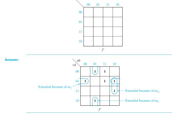
Loop the remaining 1's and write the minimum sum of products for f'.
