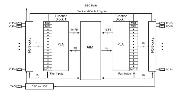
FIGURE 16-12 CoolRunner-II Architecture<sup>1</sup> (Figure based on figures and text owned by Xilinx, Inc., Courtesy of Xilinx, Inc. © Xilinx, Inc. 1999–2003. All rights reserved.)
