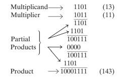
The multiplication of two 4-bit numbers requires a 4-bit multiplicand register, a 4-bit multiplier register, and an 8-bit register for the product. The product register
