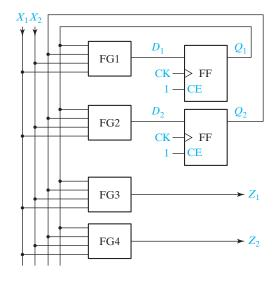
$(X_1, X_2, Q_1, \text{and } Q_2)$ . If more flip-flops or inputs are needed, the *D* or *Z* functions may have to be decomposed to use additional function generators as in Figure 9-40.
