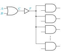
at the buffer output, this is a noninverting buffer, and the logic values of the buffer input and output are the same, that is, F = C.
