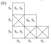
Maximal Compatibles:  $(S_0, S_1)$ ,  $(S_1, S_2)$ ,  $(S_0, S_3)$ .  $(S_0, S_3)$  and  $(S_1, S_2)$  produce a two-state reduced table.
