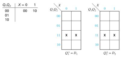
Starting with the equations for assignment A, replace all of the 1's with 2's and all 2's with 1's. Verify that the resulting equations are the same as those for assignment B.
