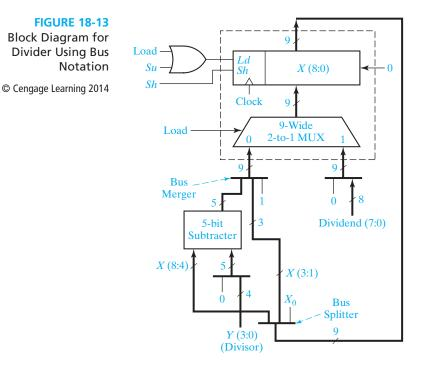
represents a *bus splitter* that splits the 9 bits from the X register into  $X_8X_7X_6X_5X_4$  and  $X_3X_2X_1$ ;  $X_0$  is not used. Bus mergers and splitters do not require any actual hardware; they are just a symbolic way of showing bus connections.
