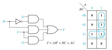
Figure 8-10(a) shows a circuit with several 0-hazards. The product-of-sums representation for the circuit output is
