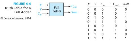
Figure 4-4 gives the truth table for a full adder with inputs X, Y, and  $C_{in}$ . The outputs for each row of the table are found by adding up the input bits  $(X + Y + C_{in})$  and splitting the result into a carry out  $(C_{i+1})$  and a sum bit  $(S_i)$ . For example, in the 101 row  $1 + 0 + 1 = 10_2$ , so  $C_{i+1} = 1$  and  $S_i = 0$ . Figure 4-5 shows the implementation of the full adder using gates. The logic equations for the full adder derived from the truth table are
