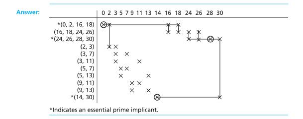
Note that all remaining columns contain two or more X's. Choose the first column which has two X's and then select the prime implicant which covers the first X in that column. Then, choose a minimum number of prime implicants which cover the remaining columns in the chart.
