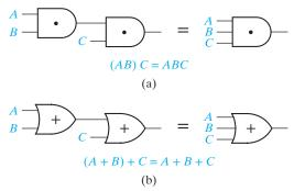
When two or more variables are ANDed together, the value of the result will be 1 if all of the variables have the value 1. If any of the variables have the value 0, the result of the AND operation will be 0. For example,
