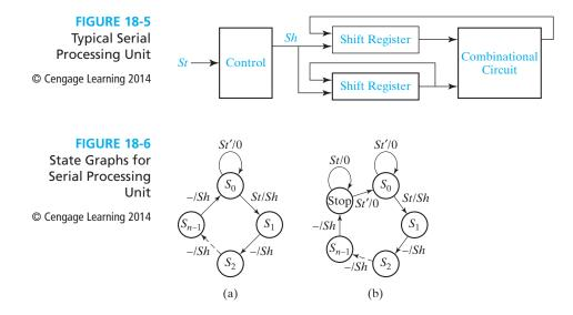
have *n* bits, then a total of *n* shift signals must be generated. If *St* is 1 for only one clock time, then the control state graph (Figure 18-6(a)) stops when it returns to state  $S_0$ . However, if *St* can remain 1 until after the shifting is completed, then a separate stop state is required, as shown in Figure 18-6(b). The control remains in the stop state until *St* returns to 0.
