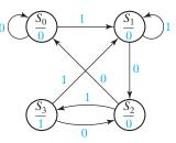
The state table corresponding to the circuit is given by Table 14-3. Note that there is a single column for the output because the output is determined by the present state and does not depend on X. Note that in this example the Moore machine requires one more state than the Mealy machine which detects the same input sequence.
