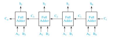
Next, we specify the FullAdder as a component within the architecture of Adder4 (Figure 10-12). The component specification is very similar to the entity declaration for the full adder, and the input and output port signals correspond to those declared for the full adder. Following the component statement, we declare a 3-bit internal carry signal C.
