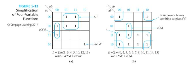
In Figure 5-12(b), note that the four corner 1's span the b = 0 columns and d = 0 rows and, therefore, can be combined to form the term b'd'. The group of eight 1's covers both rows where c = 1 and, therefore, represents the term c. The pair of 1's which is looped on the map represents the term a'bd because it is in the ab = 01 column and spans the d = 1 rows.
