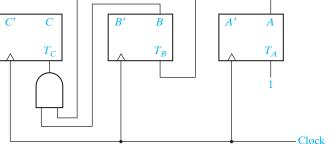
Because A changes state on every rising clock edge,  $T_A$  must equal 1. Next, observe that B changes state only if A = 1. Therefore, A is connected to  $T_B$  as shown, so that if A = 1, B will change state when a rising clock edge occurs. Similarly, C changes state when a rising clock edge occurs only if B and A are both 1. Therefore, an AND gate is connected to  $T_C$  so that C will change state if B = 1 and A = 1 when a rising clock edge occurs.
