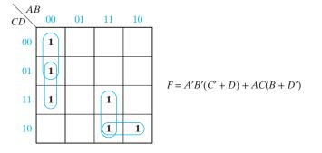
When simplifying a function algebraically, the Karnaugh map can be used as a guide in determining what steps to take. For example, consider the function
