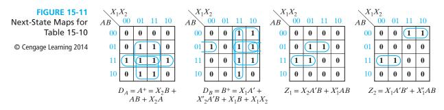
If J-K, T, or S-R flip-flops are used, the flip-flop input maps can be derived from the next-state maps using the techniques given in Section 12.6. As an example, the S-R equations for Table 15-10 are derived in Figure 15-12. The  $S_A$  and  $R_A$  maps are derived from the  $A^+$  map by applying Table 12-5(c) to the A = 0 and A = 1 halves of the map.  $S_B$  and  $R_B$  are derived in a similar manner.
