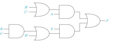
Since the output gate is an OR, the circuit can be converted to NAND gates without increasing the number of levels; Figure 7-19 is the result. Note that the three-level OR with inputs B' and C' and the four-level AND with inputs B and C both become a NAND with inputs B and C; hence, both can be replaced by the same gate.
