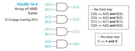
Figure 10-4 shows an array of four AND gates. The inputs are represented by bitvectors A and B, and the outputs by bit-vector C. Although we can write four VHDL statements to represent the four gates, it is much more efficient to write a single VHDL statement that performs the **and** operation on the bit-vectors A and B. When applied to bit-vectors, the **and** operator performs the **and** operation on corresponding pairs of elements.
