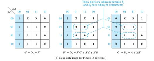
have an additional pair of adjacent 1's or adjacent 0's. This occurs because two of the three state variables are the same for adjacent assignments.
