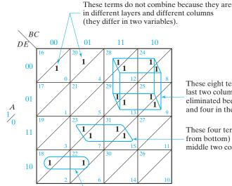
These eight terms combine to give BD'(B from last two columns and D' from top two rows; A is eliminated because four terms are in the top layer and four in the bottom).
