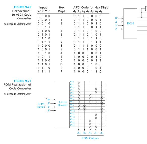
special *mask*, which is used during fabrication of the integrated circuit. Preparation of this mask is expensive, so the use of mask-programmable ROMs is economically feasible only if a large quantity (typically several thousand or more) is required with the same data array. If a small quantity of ROMs is required with a given data array, EEPROMs may be used.
