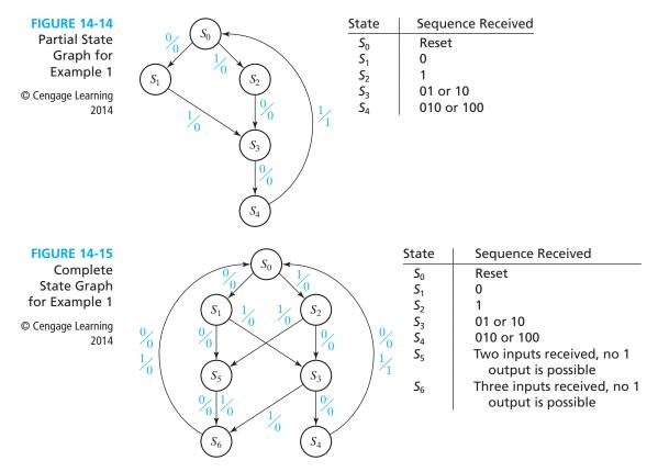
The addition of states  $S_5$  and  $S_6$  was necessary so that the circuit would not reset to  $S_0$  before four inputs were received. Note that once a 00 or 11 input sequence has been received (state  $S_5$ ), no output of 1 is possible until the circuit is reset.
