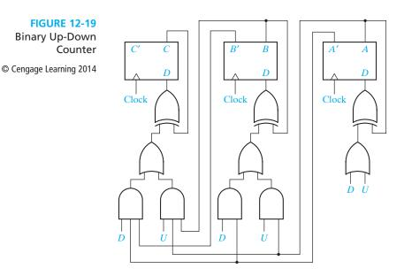
By inspection of the table in Figure 12-18, we can verify that these are the correct equations for a down counter. For every row of the table,  $A^+ = A'$ , so A changes state every clock cycle. For those rows where A = 0,  $B^+ = B'$ . For those rows where B = 0 and A = 0,  $C^+ = C'$ .
