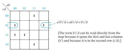
Loop two other pairs of adjacent 1's on this map and state the algebraic equivalent of looping these terms. Now read the loops directly off the map and check your algebra.
