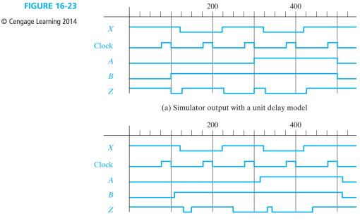
(b) Simulator output with a nominal delay of 10 ns
