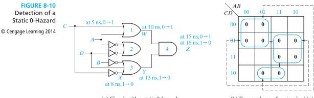
(a) Circuit with a static 0-hazard
