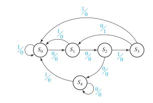
Verify that this state graph gives the proper output sequences for the input sequences listed at the start of this exercise. Write down the Mealy state table which corresponds to the preceding graph.
