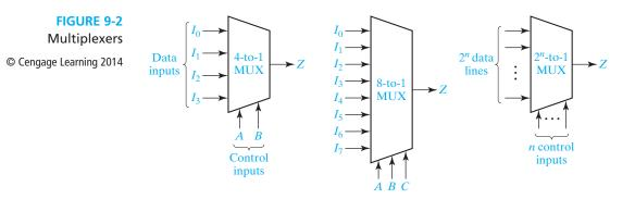
Similarly, the 8-to-1 MUX selects one of eight data inputs using three control inputs. It is described by the equation
