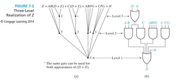
node on the tree diagram represents a gate, and the number of gate inputs is written beside each node.
