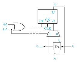
can either be loaded directly from  $y_i$  or from the sum output  $(s_i)$ . When Ld = 1 the multiplexer selects  $y_i$ , and  $y_i$  is loaded into the accumulator flip-flop  $(x_i)$  on the rising clock edge. When Ad = 1 and Ld = 0, the adder output  $(s_i)$  is loaded into  $x_i$ . The Ad and Ld signals are ORed together to enable the clock when either addition or loading occurs. When Ad = Ld = 0, the clock is disabled and the accumulator outputs do not change.
