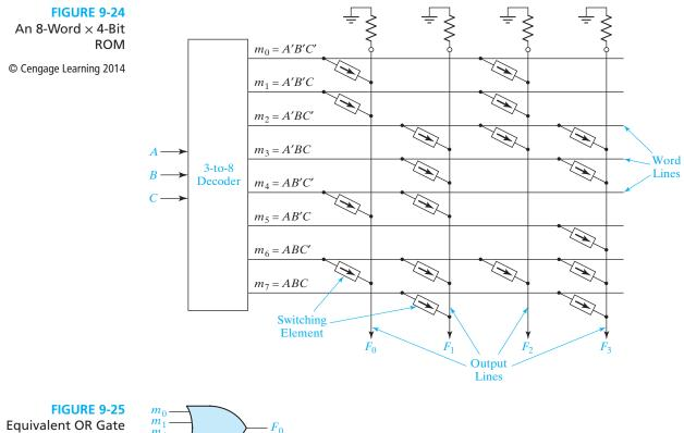
Equivalent OR Gate for  $F_0$   $m^{\dagger}$ m
