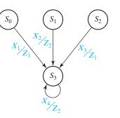
present state (PS) =  $S_0$  and  $X_1 = 1$ , PS =  $S_1$  and  $X_2 = 1$ , PS =  $S_2$  and  $X_3 = 1$ , PS =  $S_3$  and  $X_4 = 1$ . The next state of flip-flop  $Q_3$  is 1 under these four conditions (and 0 otherwise). Therefore, the next-state equation for  $Q_3$  can be written as:
