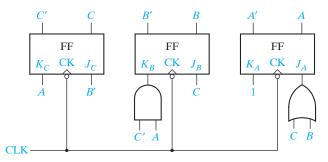
(c) Logic circuit (omitting the feedback lines)
