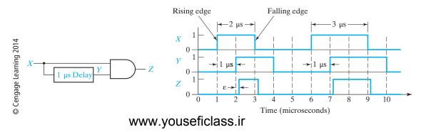
FIGURE 8-5 Timing Diagram for AND-NOR Circuit
