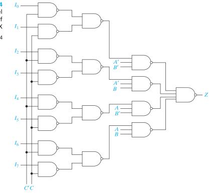
FIGURE 9-4 A Multi-Level Implementation of an 8-to-1 MUX
