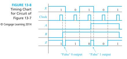
A careful interpretation of the output waveform (Z) of the Mealy circuit is necessary. After the circuit has changed state and before the input is changed, the output may temporarily assume an incorrect value, which we call a *false* output. As indicated on the timing chart, this false value arises when the circuit has assumed a new state but the old input associated with the previous state is still present.
