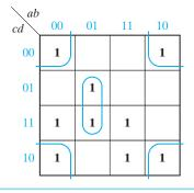
Loop the remaining 1's using a minimum number of loops. The two possible minimum sum-of-products forms for f are
