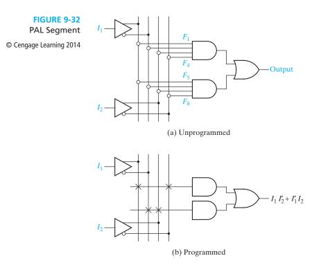
As an example of programming a PAL, we will implement a full adder. The logic equations for the full adder are
