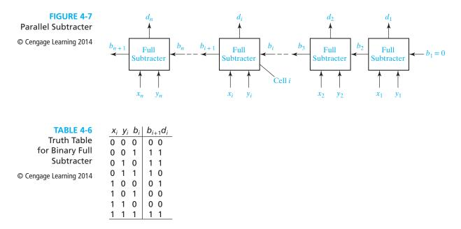
bits  $b_i$  and  $y_i$  are subtracted from  $x_i$  to form the difference  $d_i$ , and a borrow signal  $(b_{i+1} = 1)$  is generated if it is necessary to borrow from the next column.
