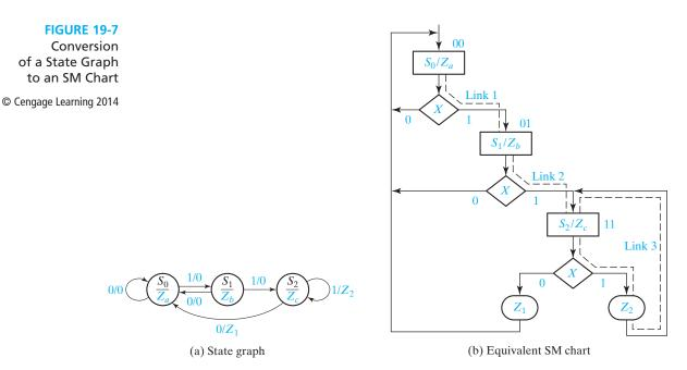
input. The Mealy outputs ( $Z_1$  and  $Z_2$ ) appear in conditional output boxes because they depend on both the state and input. In this example, each SM block has only one decision box because only one input variable must be tested. For both the state graph and SM chart,  $Z_c$  is always 1 in state  $S_2$ . If X = 0 in state  $S_2$ ,  $Z_1 = 1$  and the next state is  $S_0$ . If X = 1,  $Z_2 = 1$  and the next state is  $S_2$ .
