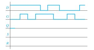
(b) Now draw in the internal signals *S* and *R* from Figure 11-14, and confirm that *S* and *R* give the same value for *Q* as in (a).
