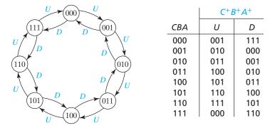
The up-down counter can be implemented using D flip-flops and gates, as shown in Figure 12-19. The corresponding logic equations are
