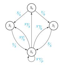
**15.35** Implement the following state graph using D flip-flops and gates. Use a one-hot assignment and write down the logic equations by inspecting the state graph.
