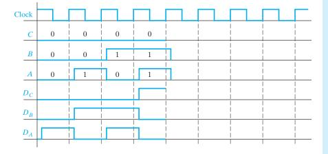
(d) Complete the following timing diagram for the binary counter of Figure 12-16.
