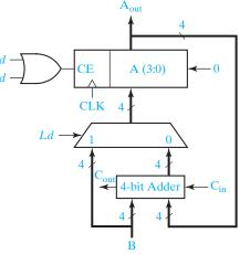
lines 11, 19, and 20 that A is a 4-bit register that changes state on the rising clock edge. It also infers the presence of a 4-wide 2-to-1 multiplexer to select either B or the adder output to load into A. Because A is loaded when Ld = 1 or Ad = 1, the CE input to the register is Ld + Ad. At this point, a block diagram of the synthesized code resembles that shown in Figure 17-25. The synthesizer output is then optimized and fit into a specific target device.
