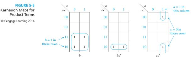
If a function is given in algebraic form, it is unnecessary to expand it to minterm form before plotting it on a map. If the algebraic expression is converted to sum-ofproducts form, then each product term can be plotted directly as a group of 1's on the map. For example, given that
