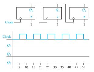
**11.25** Fill in the following timing diagram for a rising-edge-triggered T flip-flop with an asychronous active-low PreN input. Assume *Q* begins at 1.
