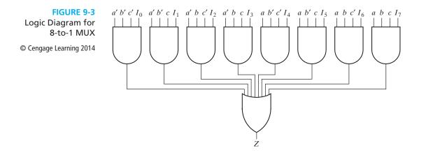
Of course, there are several other implementations of the 8-to-1 MUX. Each of the gates in Figure 9-3 can be replaced by NAND gates to obtain a NAND gate implementation. If a NOR gate implementation is wanted, the equation for Z can be written as a product of sums:
