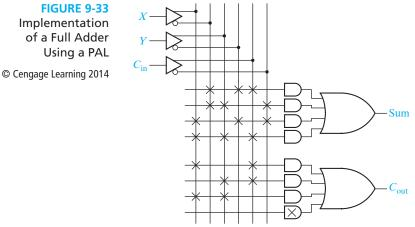
Implementation of a Full Adder Using a PAL
