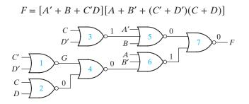
When a student builds the circuit in lab, he finds that when A = C = 0 and B = D = 1, the output *F* has the wrong value and that the gate outputs are as shown. Determine some possible causes of the incorrect output if G = 0 and if G = 1
