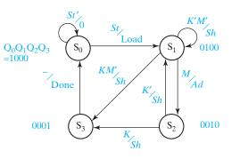
is  $S_2$ . If M = 0 and K = 0, the output is Sh = 1 and the next state is  $S_1$ . If M = 0 and K = 1, the output is Sh = 1 and the next state is  $S_3$ . In  $S_2$ , the output is Sh = 1 for both K = 0 and K = 1. If K = 0, the next state is  $S_1$ , and if K = 1, the next state is  $S_3$ . In  $S_3$ , the output is Done = 1 and the next state is  $S_0$ .
