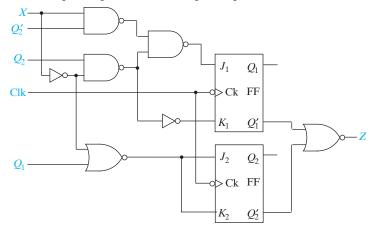
**13.21** A Mealy sequential circuit has one input, one output, and two flip-flops. A timing diagram for the circuit follows. Construct a transition table and state graph for the circuit.
