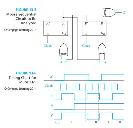
fifth rising clock edge causes the state to change to AB = 11. The input, state, and output sequences are plotted on the timing chart of Figure 13-6 and are also listed below.
