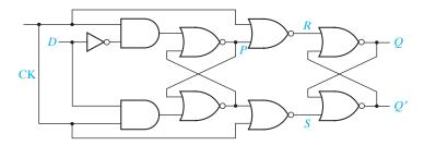
In this exercise you will be asked to analyze the operation of the D flip-flop shown above by filling in a table showing the values of CK, D, P, S, R, and Q after each change of input. It will be helpful if you mark the changes in these values on the circuit diagram as you trace the signals. Initially, assume the following signal values:
