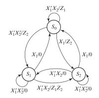
**14.46** There are two errors in the state graph shown. One state is not completely specified for one combination of  $X_1$  and  $X_2$ . In another state, there is a contradiction for one combination of  $X_1$  and  $X_2$ . Correct the state graph by making two minor changes. Demonstrate that the modified state graph is completely specified.
