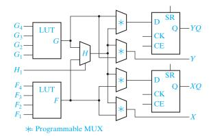
the flip-flop inputs are selected by programmable multiplexers. The select inputs to these MUXes are programmed when the FPGA is configured. For example, the X output can come from the F function generator, and the Y output from the H multiplexer. Operation of the CLB flip-flops will be described in Unit 11.
