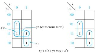
If a function has two or more minimum sum-of-products forms, all of these forms can be determined from a map. Figure 5-9 shows the two minimum solutions for  $F = \Sigma m(0, 1, 2, 5, 6, 7)$ .
