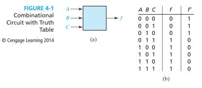
Next, we will derive an algebraic expression for f from the truth table by using the combinations of values of A, B, and C for which f = 1. The term A'BC is 1 only if A = 0, B = 1, and C = 1. Similarly, the term AB'C' is 1 only for the combination 100, AB'C is 1 only for 101, ABC' is 1 only for 110, and ABC is 1 only for 111. ORing these terms together yields
