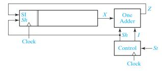
The control circuit outputs *I*, which should set the ONE ADDER to the proper initial state, and then outputs *Sh* to the shift register the required number of times. Design the box labeled "ONE ADDER" using NOR gates and a D flip-flop with preset and clear inputs.
