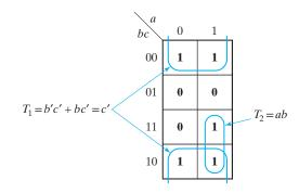
The Karnaugh map can also illustrate the basic theorems of Boolean algebra. Figure 5-8 illustrates the consensus theorem, XY + X'Z + YZ = XY + X'Z. Note that the consensus term (YZ) is redundant because its 1's are covered by the other two terms.
