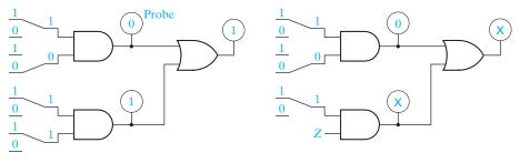
(a) Simulation screen showing switches
