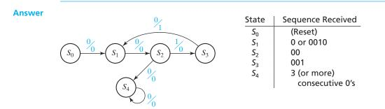
The preceding state graph is not complete because there is only one arrow leaving most states. Complete the graph by adding the necessary arrows. Return to one of the previously used states when possible.
