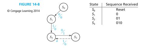
are looking. Therefore, we can go back to state  $S_2$  (arrow a) because  $S_2$  corresponds to having received a sequence ending in 01. Then, if we get another 0 in state  $S_2$ , we go to  $S_3$  with a 1 output. This is correct because the sequence again ends in 010.
