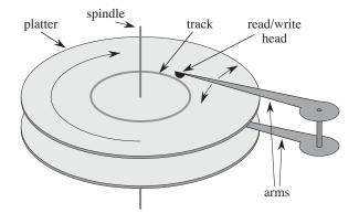
**Figure 18.2** A typical disk drive. It comprises one or more platters (two platters are shown here) that rotate around a spindle. Each platter is read and written with a head at the end of an arm. Arms rotate around a common pivot axis. A track is the surface that passes beneath the read/write head when the head is stationary.
