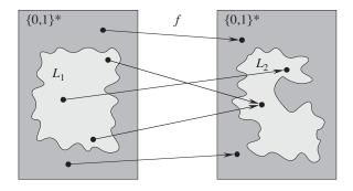
**Figure 34.4** An illustration of a polynomial-time reduction from a language  $L_1$  to a language  $L_2$  via a reduction function f. For any input  $x \in \{0, 1\}^*$ , the question of whether  $x \in L_1$  has the same answer as the question of whether  $f(x) \in L_2$ .
