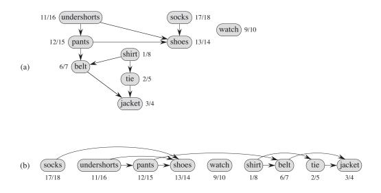
**Figure 22.7** (a) Professor Bumstead topologically sorts his clothing when getting dressed. Each directed edge (u, v) means that garment u must be put on before garment v. The discovery and finishing times from a depth-first search are shown next to each vertex. (b) The same graph shown topologically sorted, with its vertices arranged from left to right in order of decreasing finishing time. All directed edges go from left to right.
