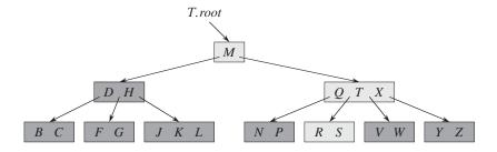
**Figure 18.1** A B-tree whose keys are the consonants of English. An internal node *x* containing x.n keys has x.n + 1 children. All leaves are at the same depth in the tree. The lightly shaded nodes are examined in a search for the letter *R*.
