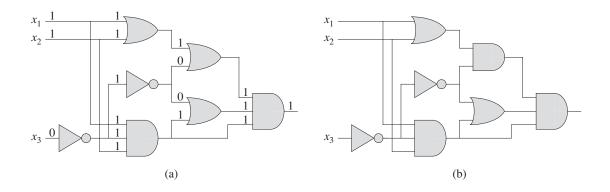
**Figure 34.8** Two instances of the circuit-satisfiability problem. (a) The assignment  $\langle x_1 = 1, x_2 = 1, x_3 = 0 \rangle$  to the inputs of this circuit causes the output of the circuit to be 1. The circuit is therefore satisfiable. (b) No assignment to the inputs of this circuit can cause the output of the circuit to be 1. The circuit is therefore unsatisfiable.
